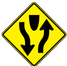
Start of Divided Highway
