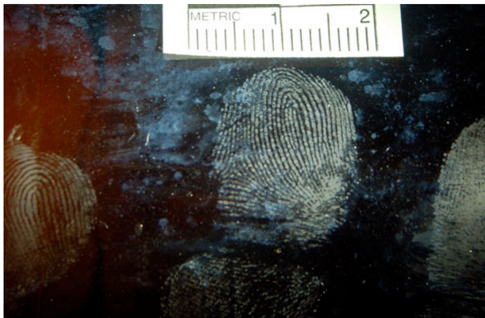
Super glue fumes adhere to latent fingerprints on the neck of a glass bottle. (Courtesy of Scott Campbell, Ron Smith & Associates)
