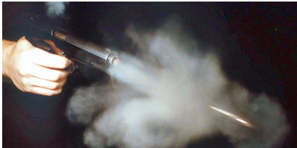
Propellants and other gunshot residues expelled during the firing process. (Courtesy of Jack Dillon)
