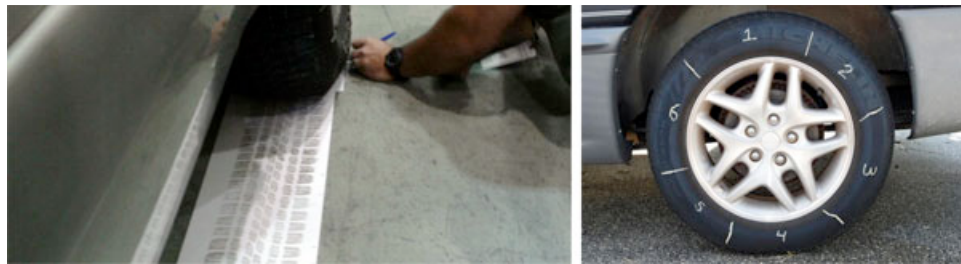
A reference print from a tire is captured by inking the tire and driving over paper. (Courtesy of John Black, Ron Smith & Associates)
