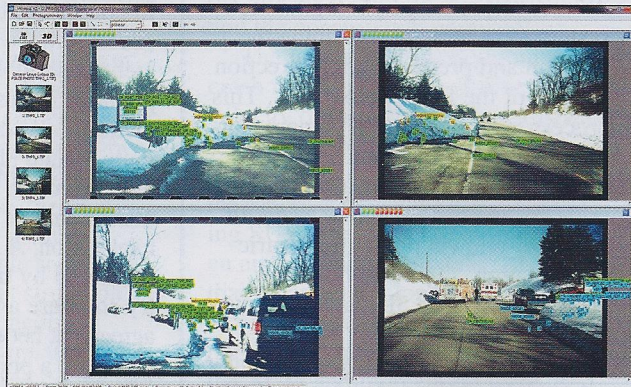
Figure 4 —Four police photos were utilized in this reconstruction, as seen here in the iWitness photogrammetry software interface.
