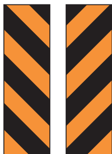
Hazard to left Hazard to right
